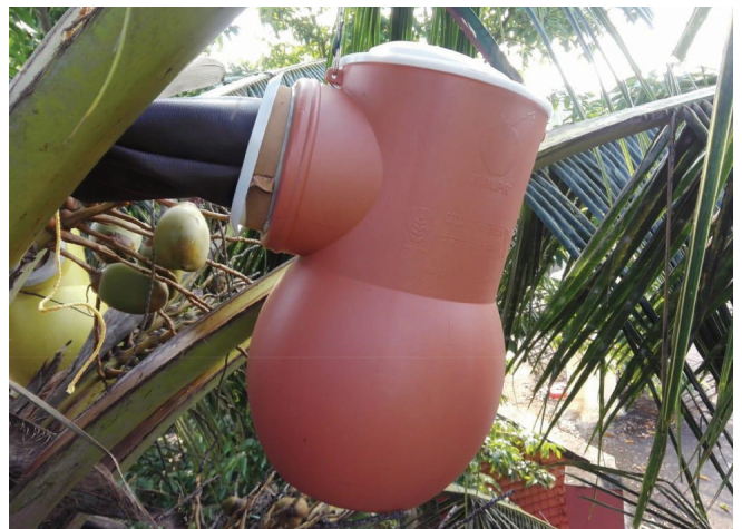
Fig. 5: Coco-sap chiller developed by ICAR-CPCRI for the collection of unfermented coconut inflorescence sap.
