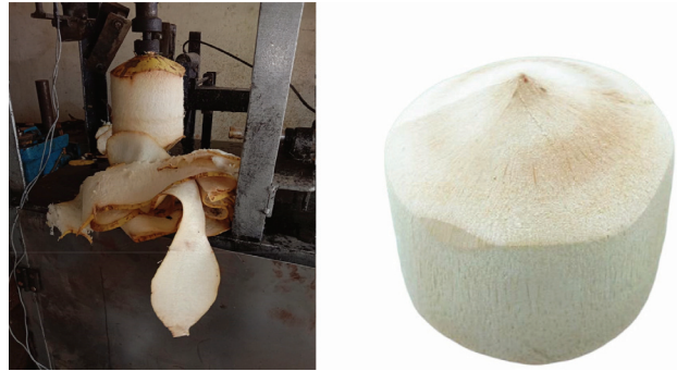
Fig. 9: Trimming Machine for the production of minimally processed tender nuts
