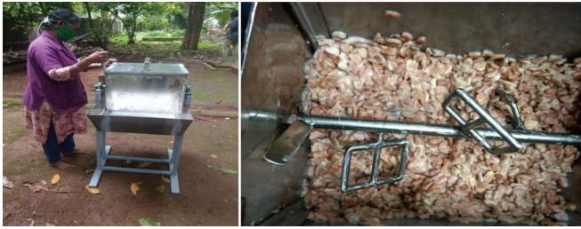
Fig. 16: Cocoa bean fermentor developed at KAU
